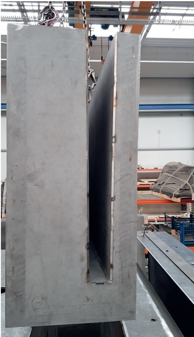
Interchangeable insert for the core to form the inner walls of a station
