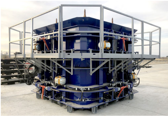
MT20 dry cast box culvert machine
