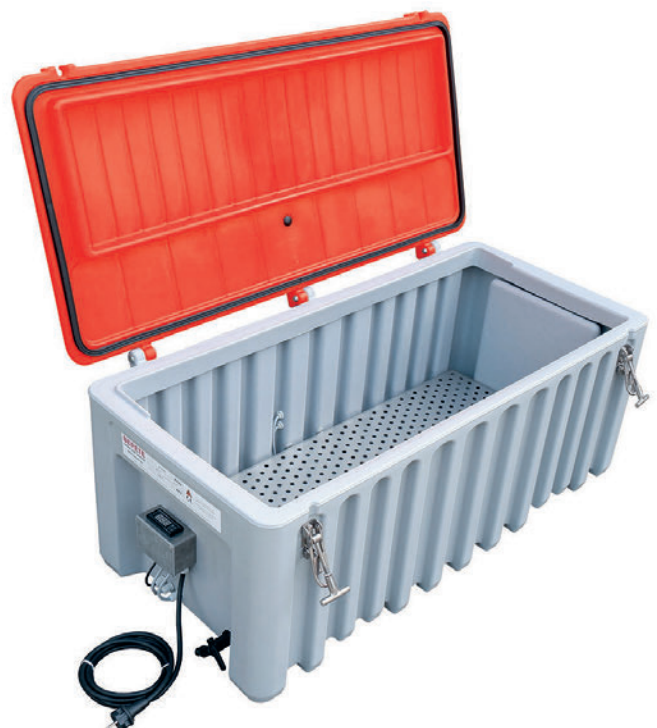
Plastic concrete sample curing tank
