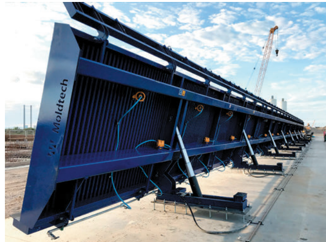
Tilting table for the production of sound walls
