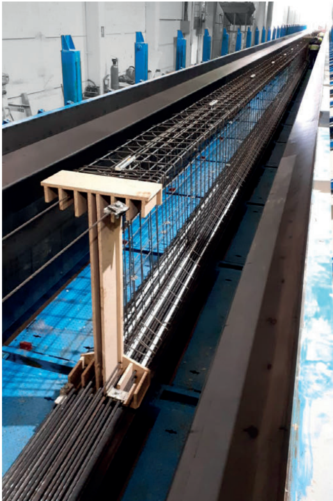
The automated, highly flexible mould for manufacturing beams was designed especially for Hormipresa
