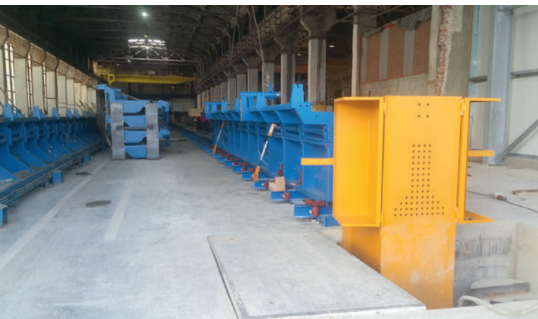
View of the fixed abutment
