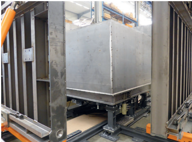
Assembled formwork for transformer substations on site
