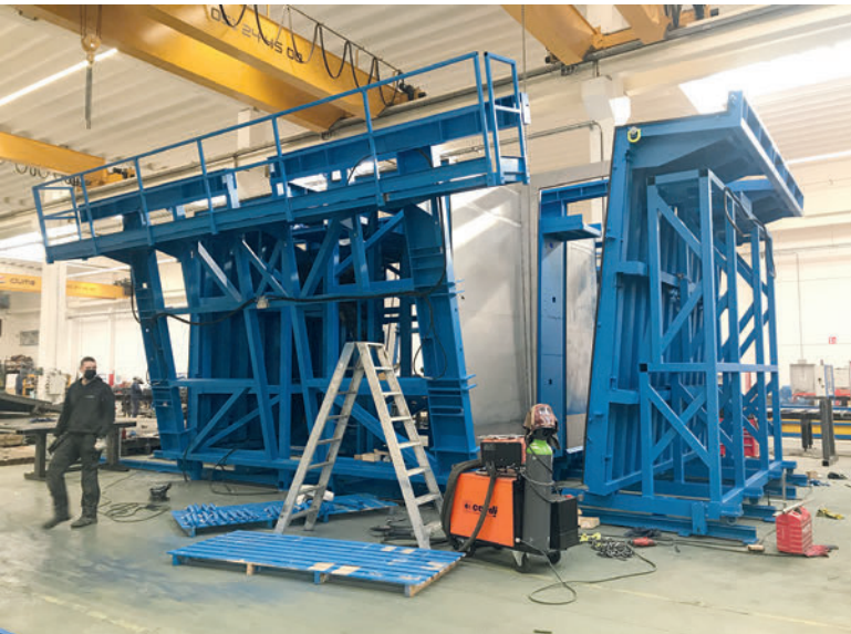
Fig. 6: Fully hydraulic quadruple mould with stainless steel sheeting
