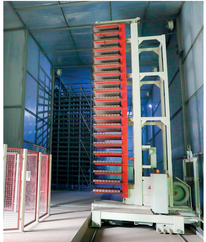
Finger car, 14to capacity
