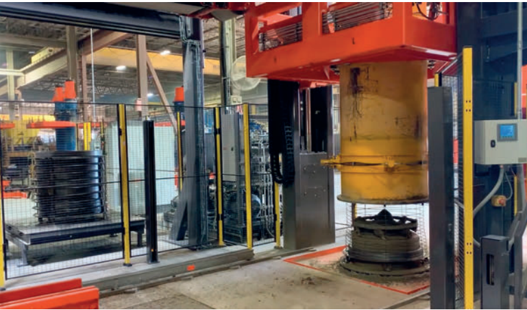
The Mastermatic XT150 is a self-stripping machine and does not require an overhead crane.
