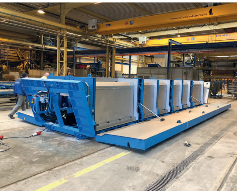
Fig. 4: Fully hydraulic mould with stainless steel sheeting
