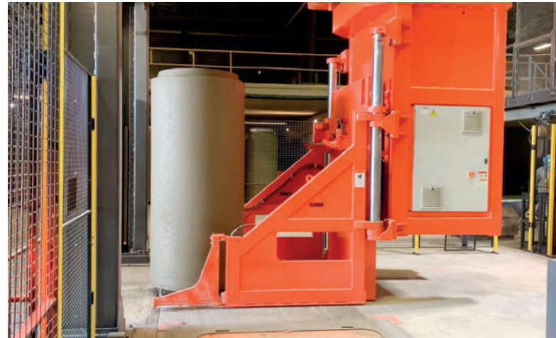
Offbearing device removing the pipe and placing it for transport to the kiln.
