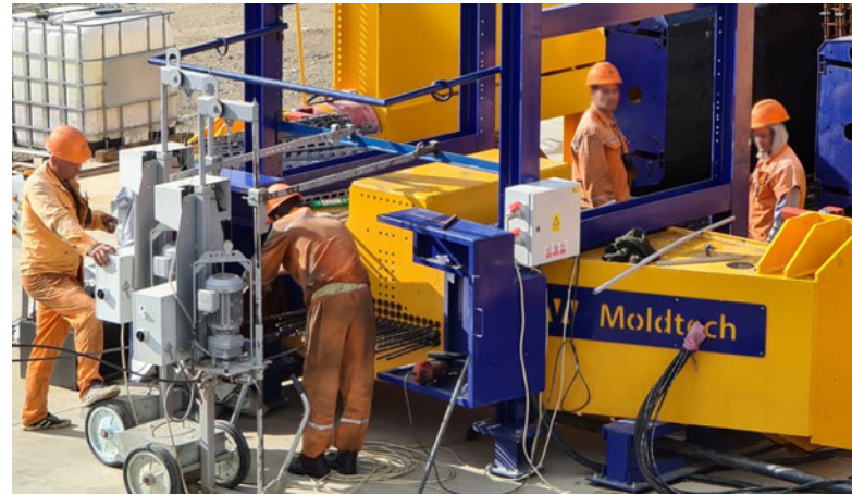
Active self-stressing head for 1500 Tn of pre-stress
