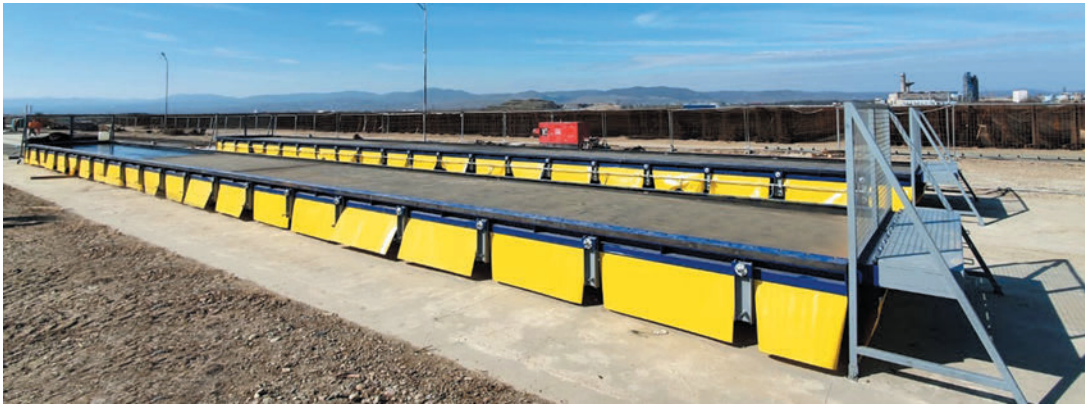
Fixed table for the production of half slabs
