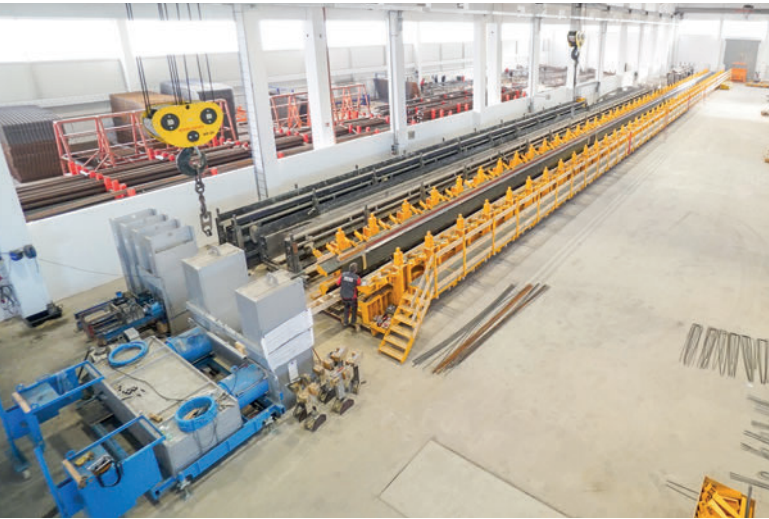
72.00 m Howal Hystanplus type 220 beam formwork
