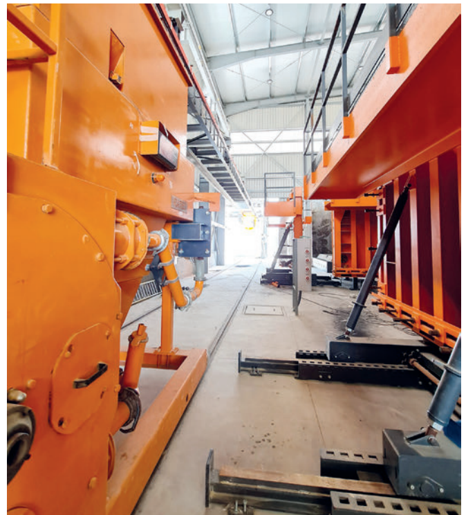
The pump car provides the individual moulds via rail tracks with concrete from the mixing plant.
