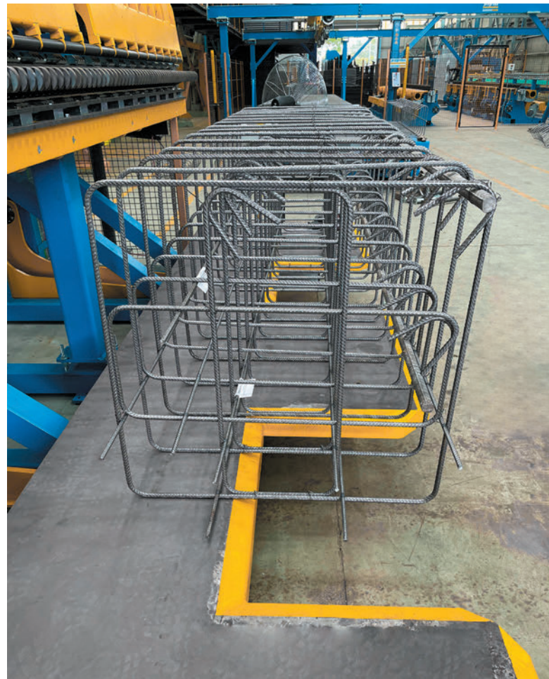
Finished rebar labelled and prepared for transport to be used in precast elements by Euro Precast.
