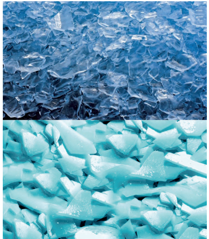
Plate ice (top) and flake ice (bottom), as classic types of ice for concrete cooling. Plate ice can be produced approx. 30 - 45 per cent more energy-efficiently
