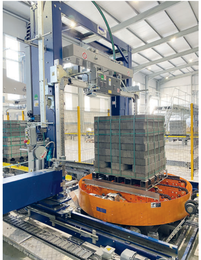
A cube of voided UK concrete coursing brick (with horizontal and two side vertical strapping) leaves the Stowell strapping line on a slave strapping pallet.
