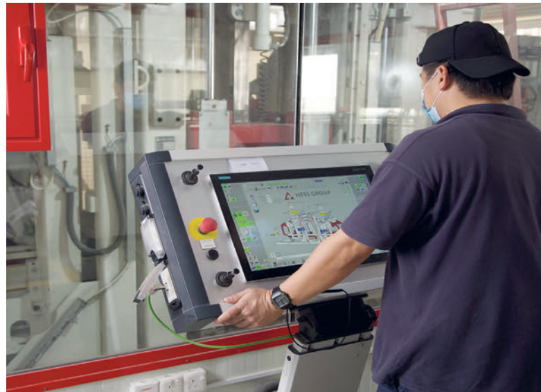
Like all concrete block machines produced by the Hess Group, the new unit at Artic is also equipped with an operating console.
