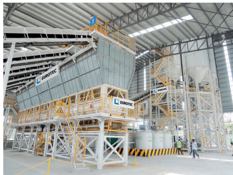
The Eurotec MZP200 concrete plant features a modularised structure for easy and quick installation and maintenance.
