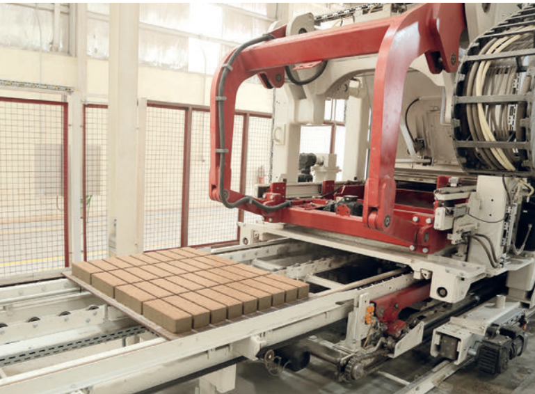
Production is done on 1,400 x 1,100 x 14 mm steel production boards.
