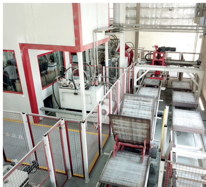
Cross conveyor with board turnover device and board buffer conveyor; in the background the magnetic stacking device
