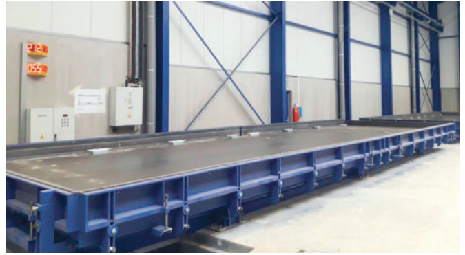
Tilting tables with LED displays for frequency controlled vibration
