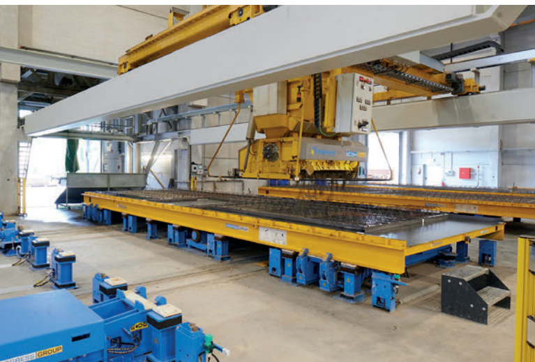
Concreting and compaction station
