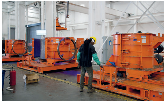
The Prima process line brings the forms to the worker saving steps and reducing the labor input per piece.
