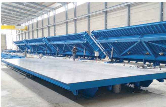
Overview of precast production facility with tilting tables
