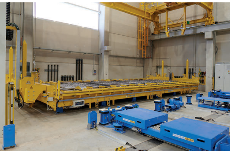
Turning device and clamping of the 1 st shell for the double wall
