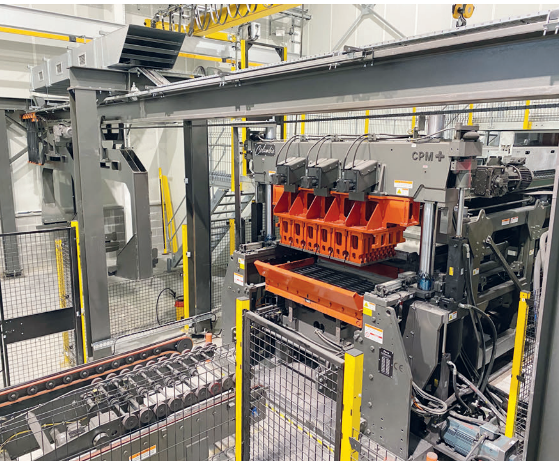
Twin cassette fully automatic mould change inside a generous CDS sound room with 2.5 tonne overhead crane and targeted dust extraction.
