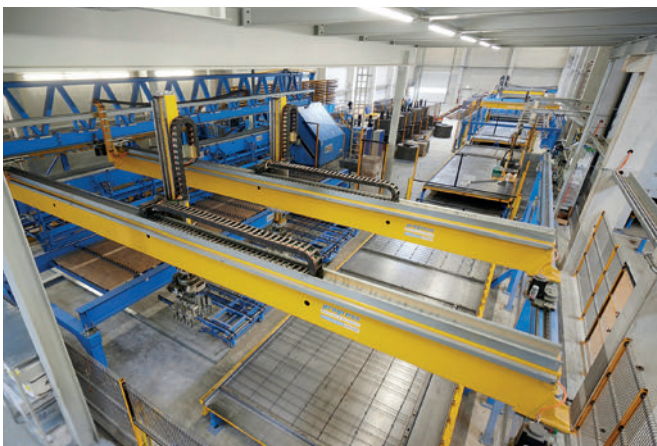
Automatic laying of reinforcement with double insertion robot
