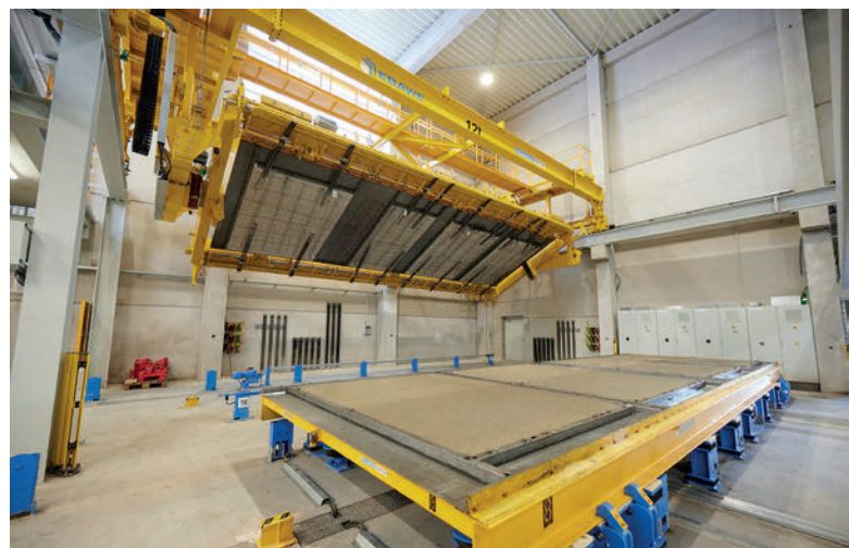
Turning of the double wall
