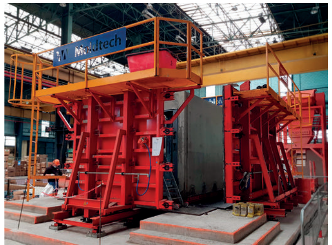
Demoulding of casted element
