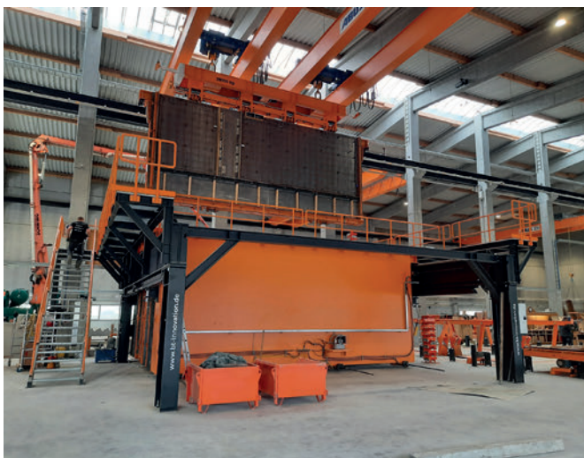
Insertion of a Butterfly Formwork into the Butterfly Battery Mould
