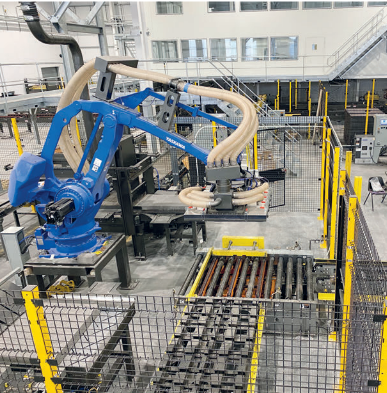
Vacuum product cubing robot with Columbia slave pallet strapping and hooding circuit.
