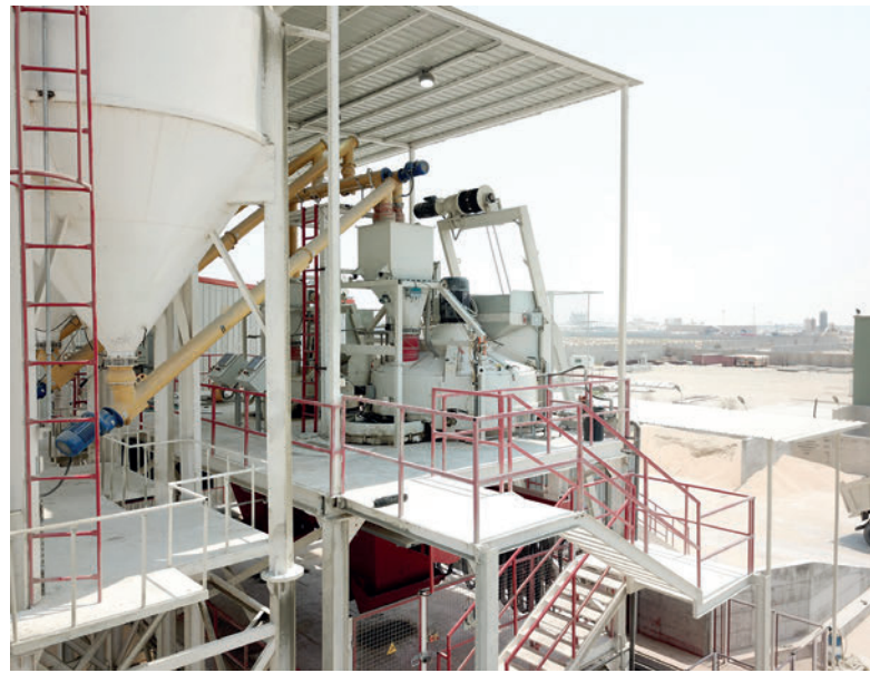
Two planetary mixers were selected for the concrete production: the large SX3750 for the core concrete and the smaller SX750 for the facing concrete.
