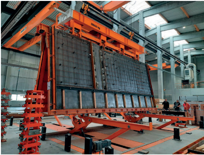
Smooth folding up the formwork with special hydraulic equipment
