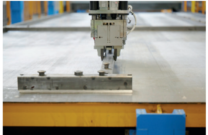
Shuttering robot and patented centimetre shuttering
