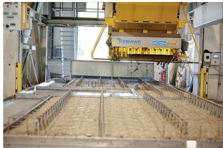
Automatic concrete discharge
