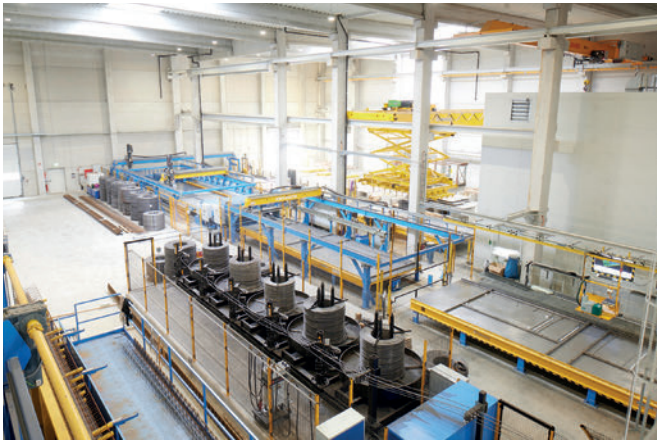
Shuttering logistics with three robots
