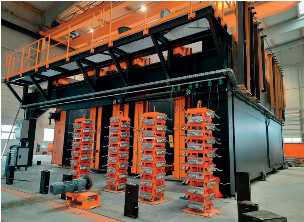
Butterfly Battery Mould with MagFly magnets
