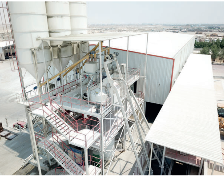
Two planetary mixers were selected for the concrete production: the large SX3750 for the core concrete and the smaller SX750 for the facing concrete.
