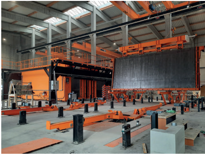
Patented Butterfly Battery Mould combines the advantages of horizontal preparation and vertical production
