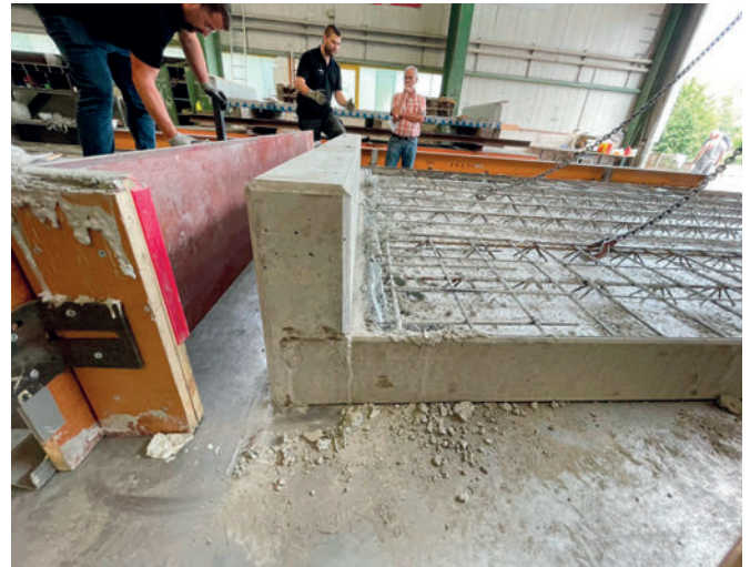
Easier production of upstands in solid elements with significant reduction in formwork timber.
