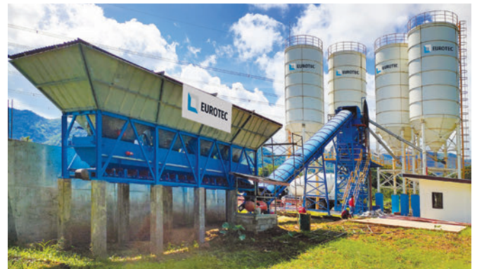
In Batangas, Philippines a Eurotec ECO90 concrete batching plant has been supplying ready-mix concrete for commercial projects.
