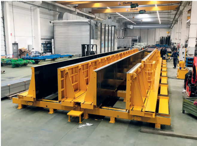
Bibat mould 18m long, with interchangeable panels and box-outs for corbels
