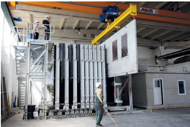
Typical necessary machinery and equipment for prefabrication of large panel-shaped elements
