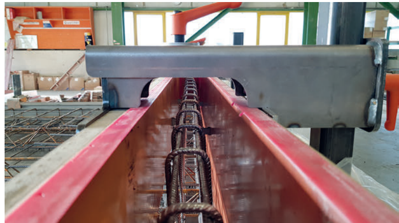
The universal plywood beam has now been supplemented by an extension arm for the production of solid upstands.
