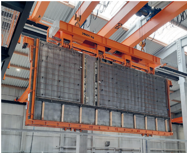
Butterfly formwork® and battery mould, combination of horizontal preparation with vertical casting
