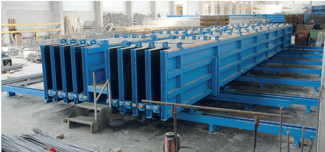
Multibat mould, 16m long, with 8 pockets 1250mm high
