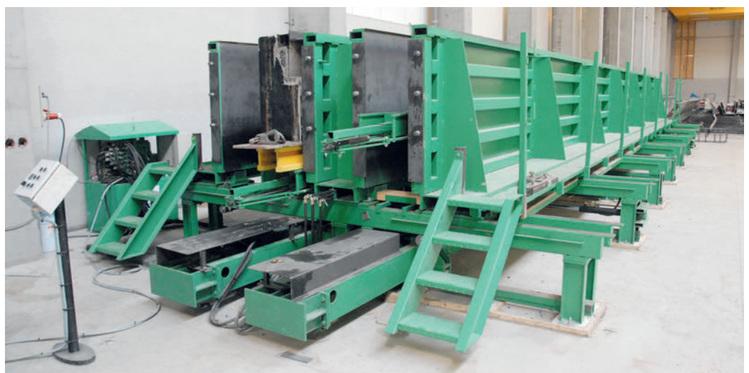
Bibat hydraulic battery mould 14m long, with hydraulic height adjustment system
