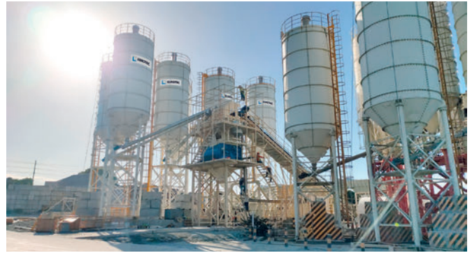
The PTT120 concrete plant is designed in modules for enhanced portability and easy transportation.
