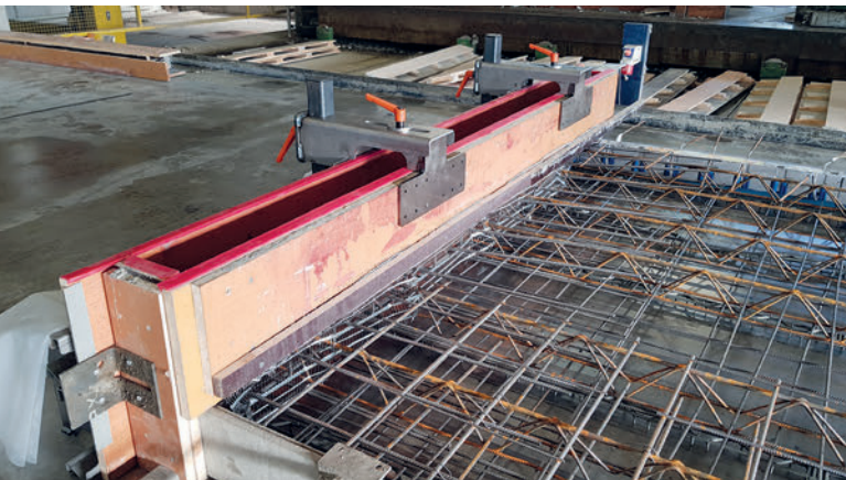
The universal plywood beam has now been supplemented by an extension arm for the production of solid upstands.
