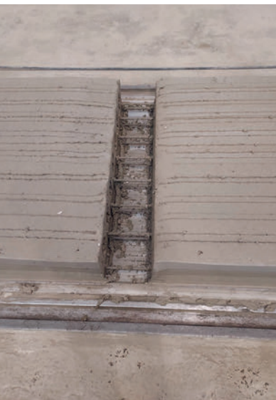
a) The 6-screw fixing system mold in standard execution and b) modified to produce the pre-stressed concrete slabs with tracks of exposed wire at both ends.
