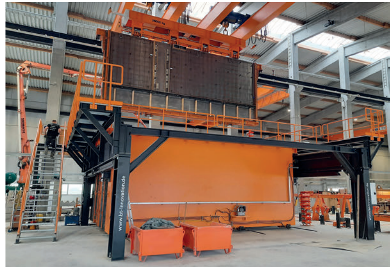
Butterfly formwork® and battery mould, combination of horizontal preparation with vertical casting
