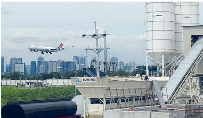
The PTT120 plant produced high-quality concrete for a two-year project at the Manila International Airport.
