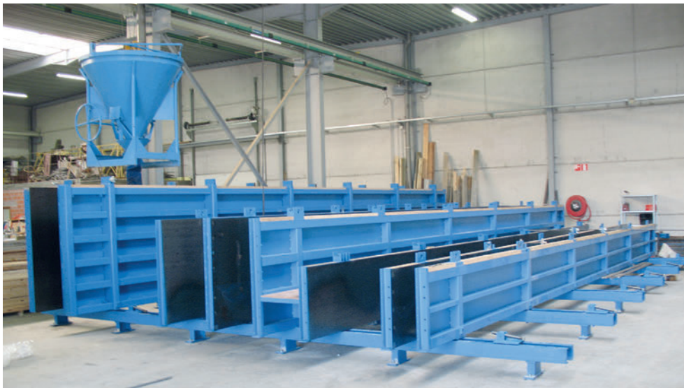
Multibat manually adjustable battery mould, 12m long, with pockets of three different heights
