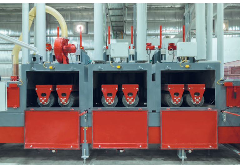
In total, the concrete stone layers or slabs pass through 6 brushes.
