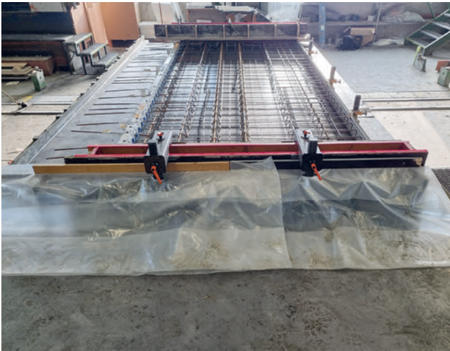
Easier production of upstands in solid elements with significant reduction in formwork timber.
