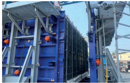
Hydraulic closing of the mould
