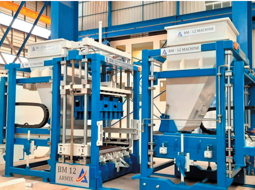
BLOCK PLANT - BM 12
