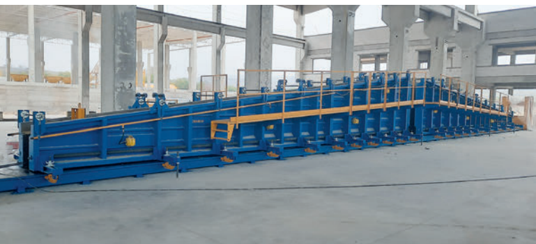
Mould sides for double slope beams
