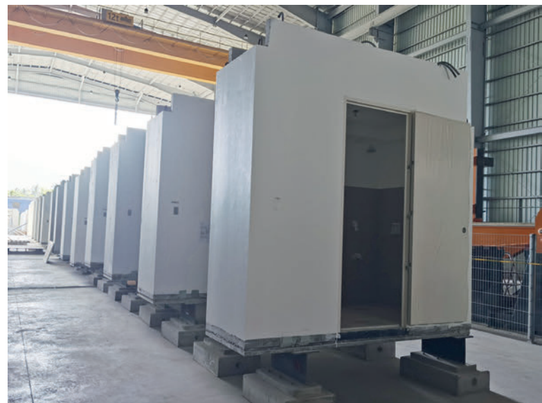
Four moulds of the flexible 3D mould kit were installed for the production of PBU (Prefabricated Bathroom Units).
