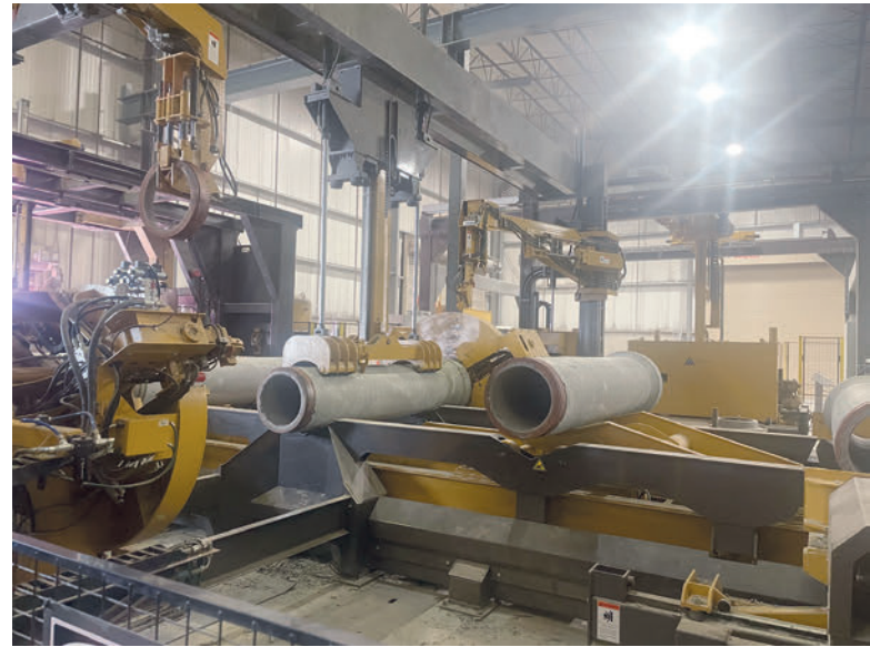
Pipe begins the Roco automated finishing process. Roco handling equipment automates the removal of the pallet and header from the finished product, stacks the joint rings, and places the product on a conveyor for further processing or transport outdoors.
