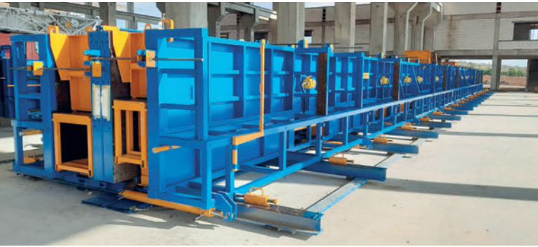
Double mould for columns
