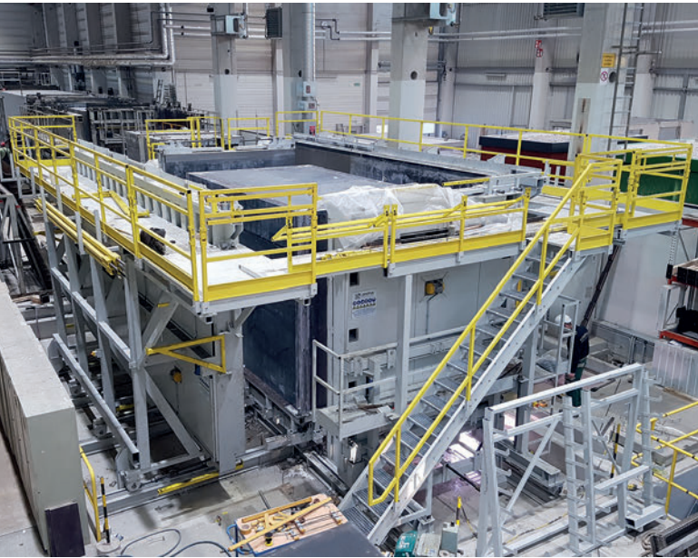
PLC controlled fully hydraulically and electrically adjustable mould
