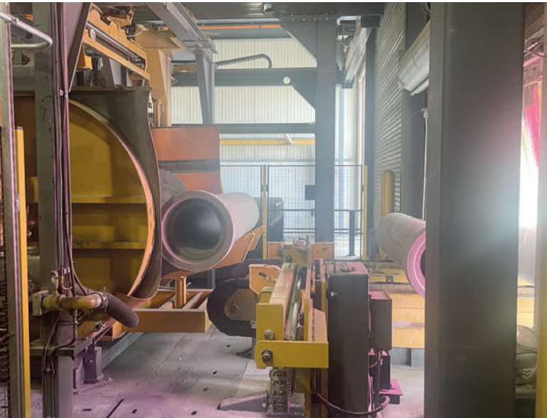
Pipes coming out of the vacuum tester.
