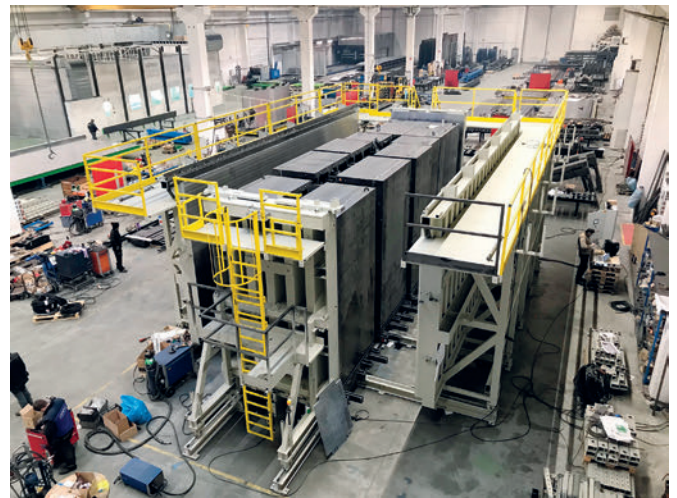
Fully adjustable substation mould in one of the Construx production facilities
