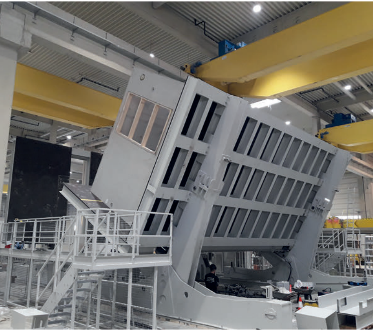
Fully automated 180° turning station with 65T capacity
