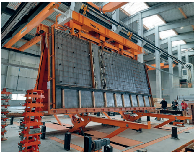
Butterfly Formwork when folded up
