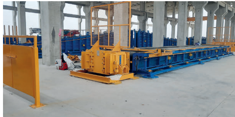
Self-reacting mould for TT slabs
