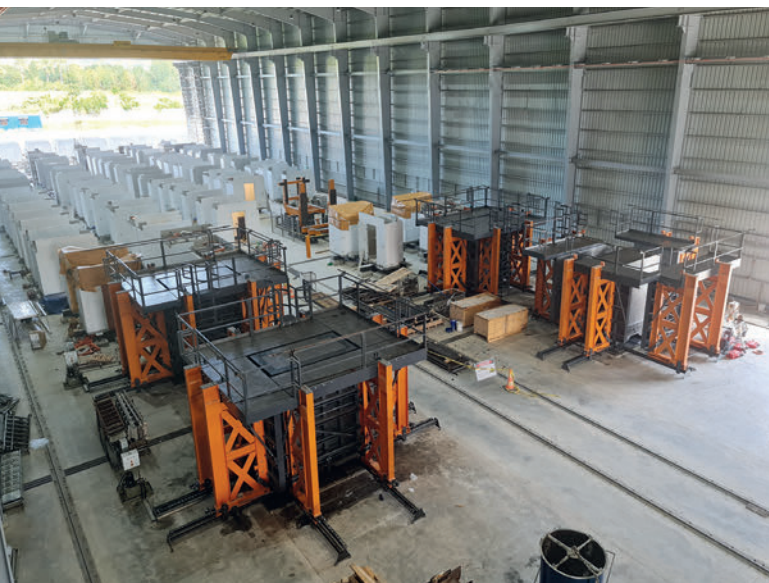
Four moulds of the flexible 3D mould kit were installed for the production of PBU (Prefabricated Bathroom Units).
