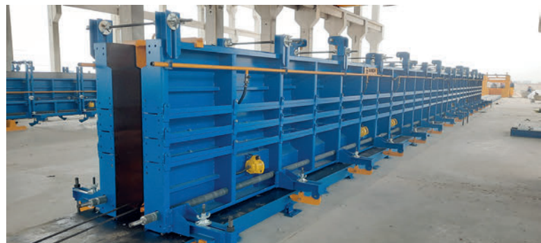
Mould sides for I beams
