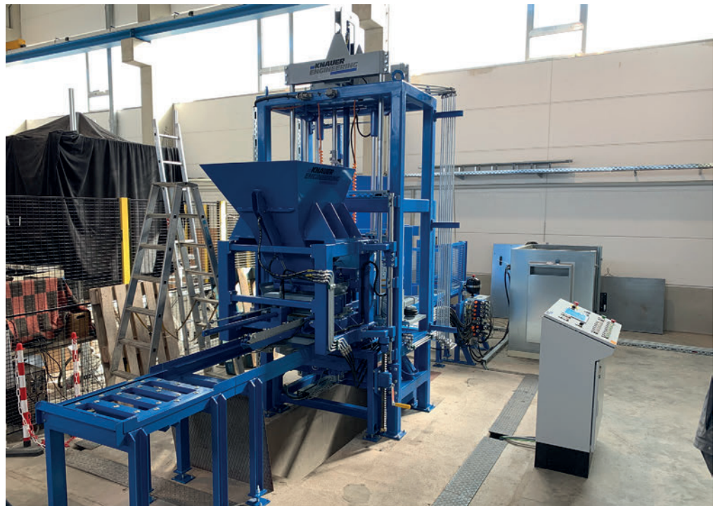
Fig. 5: Mould and compaction system immediately after set-up
