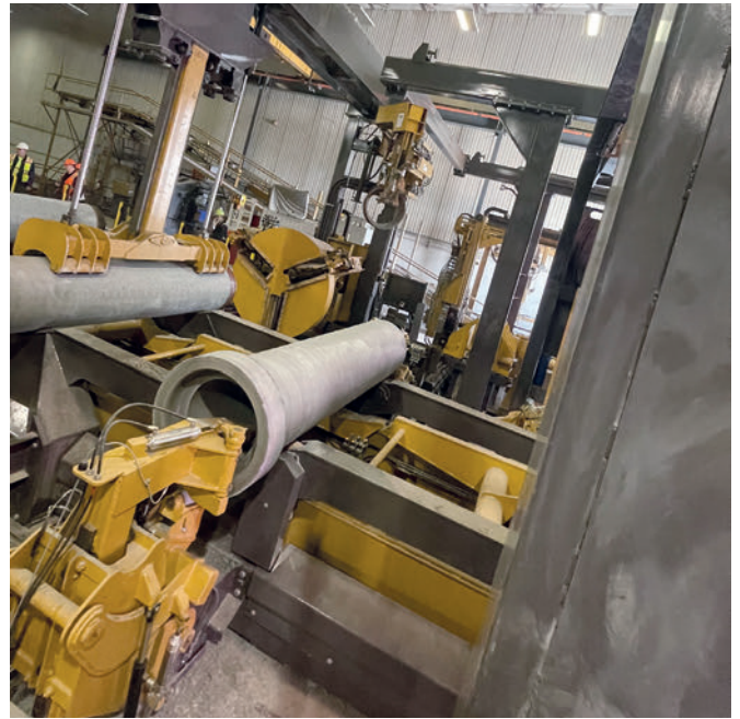
The bell and spigot end of the pipe are automatically deburred. Rotating cones deburr both the inner and outer edges of the pipe. The deburrers automatically adjust to the pipe diameter entering the system.
