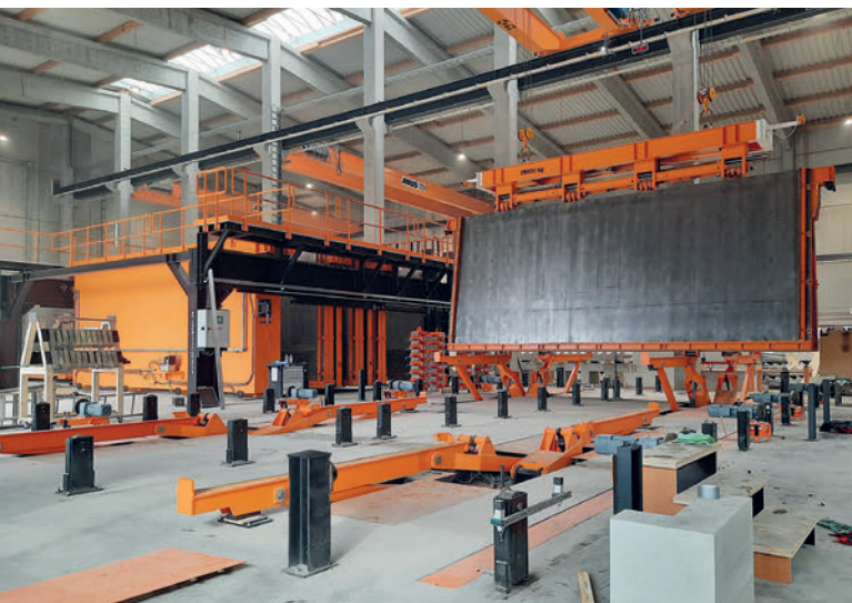
Patented Butterfly Battery® Mould combines the advantages of horizontal preparation and vertical production
