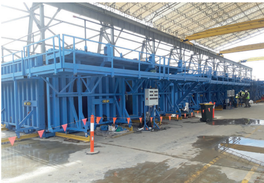
Large series of quadruple and double prison cell moulds in Grafton, Australia
