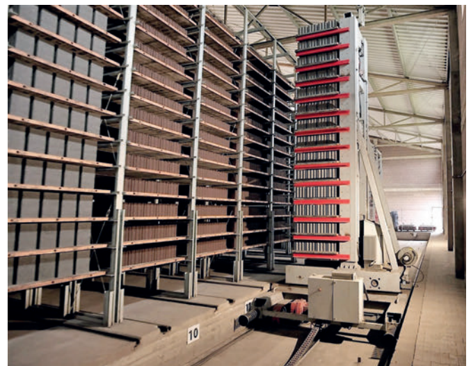
Finger car in the curing chamber
