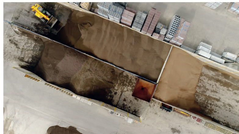
Expanded clay in different fractions from 0-4 mm to 10-20 mm.
