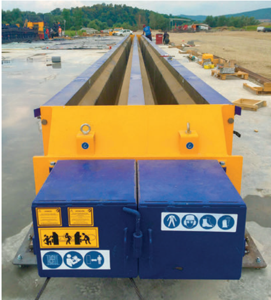
Battery mould for prestressed joist beam
