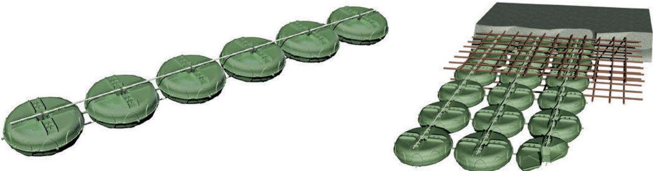
Fig. 1: Void former element Unidome XS and installed elements in a reinforced concrete slab
