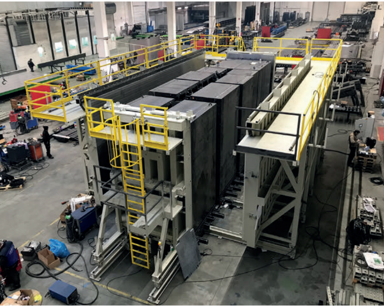
PLC controlled fully hydraulically, and electrically adjustable mould being tested in one of the Construx production facilities
