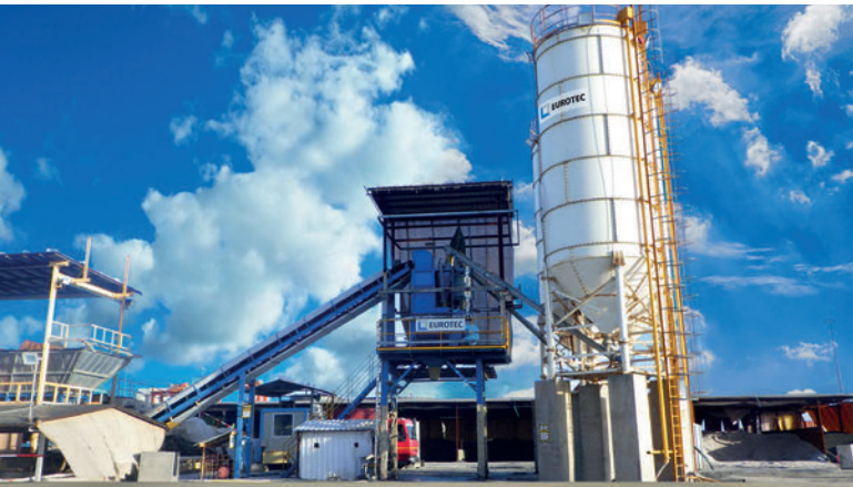
This Eurotec ECO60 Concrete Batching Plant was used by a Japanese contractor for the redevelopment of the Toamasina Port project.
