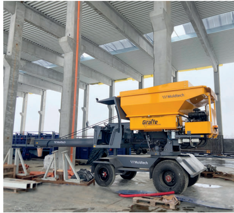
Concrete distribution vehicle Giraffe
