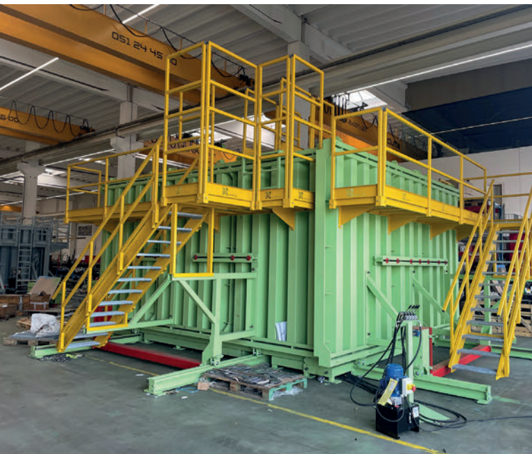
Fully adjustable box mould, ready for commissioning before leaving for Adelaide, Australia
