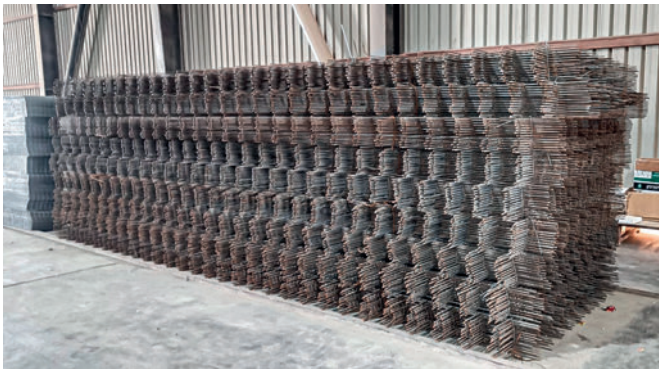
The flexible tailor-made reinforcement for the precast elements can be produced fully automated with the new machinery.
