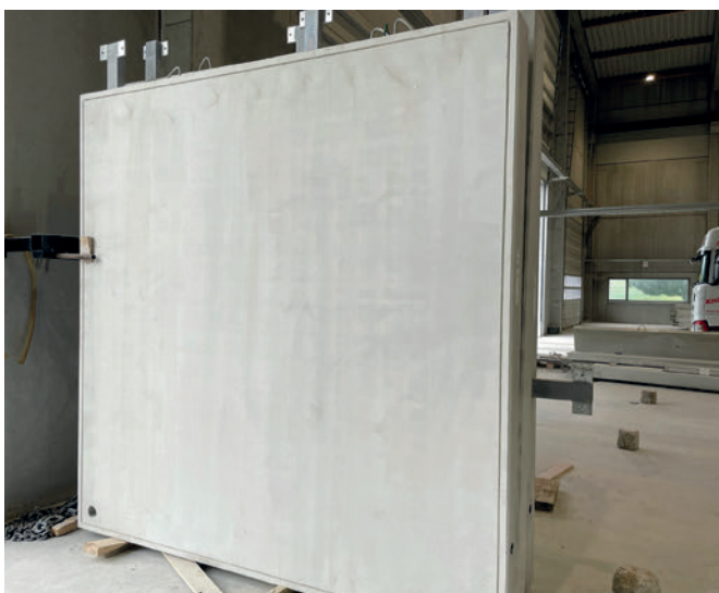
Smooth formwork surfaces on all five sides, on the edges and on the face of the recesses
