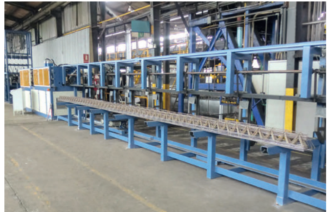
PL TRIS machine with loop accumulator and collector for lattice girders up to 15m
