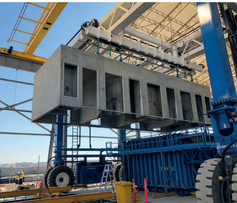
Demoulding of a quadruple prison cell unit in Grafton, Australia
