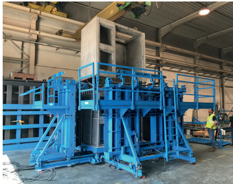
Test pour demoulding of a substation in a Construx production facility, before leaving for The Netherlands
