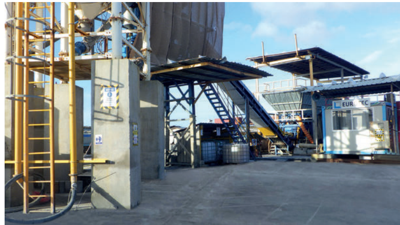
The Eurotec ECO60 can produce up to 60 m 3 /hour of ready-mix concrete in batches of 1 m 3 .
