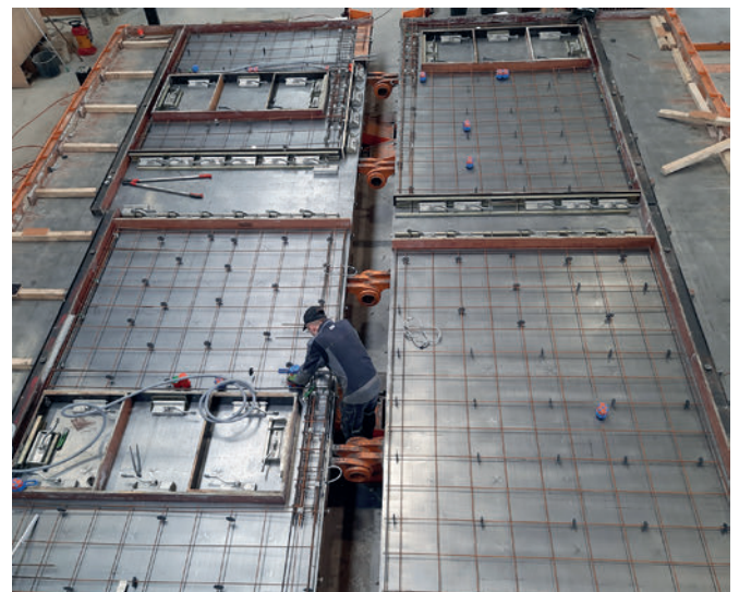
Butterfly formwork® in unfolded position - Horizontal preparation
