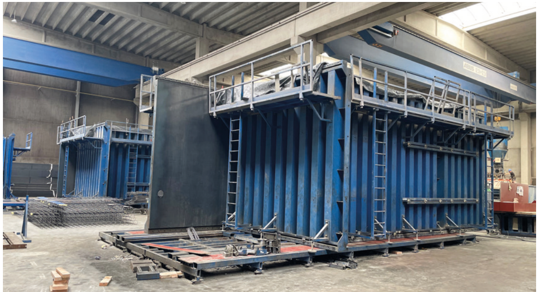
Typical setup of a Flexbox mould
