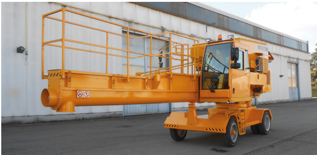
Concrete distribution machine Speedy from 2014
