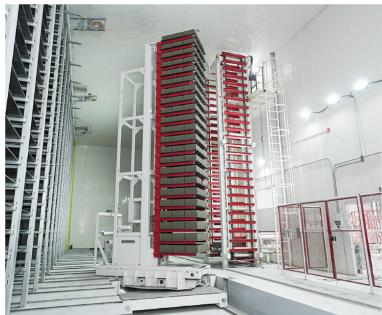
Finger cart system and curing chamber
