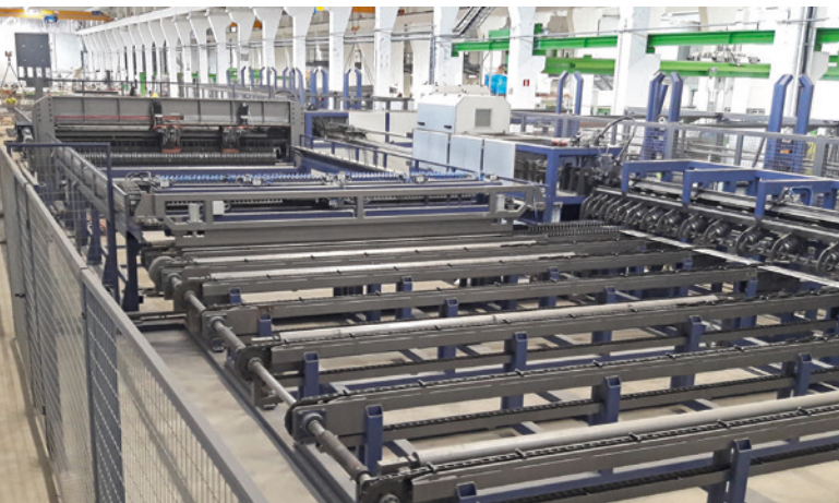
View of a PLXY AMM machine with two moving, multi-point welding heads
