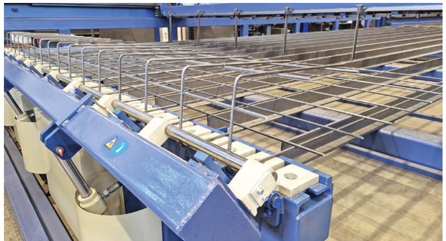
Cage production with integrated, in-line mesh bender
