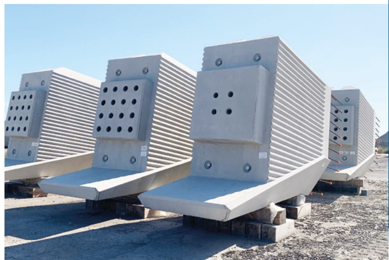
Precast bridge piers
