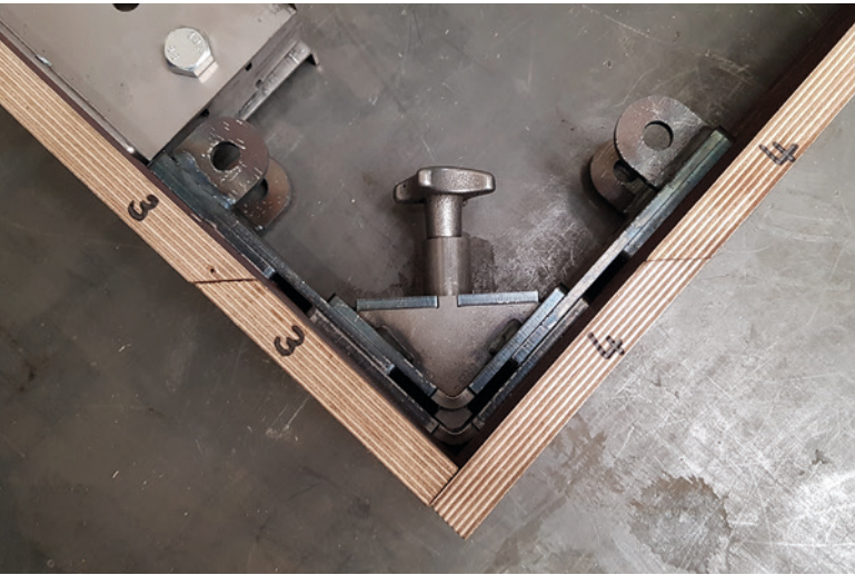
Corner bracket for planking with wood for shuttering recesses
