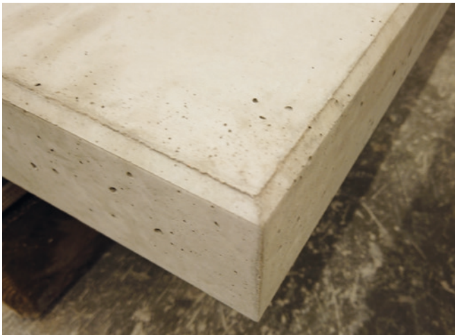
Shrink formwork suitable for robot concreting on both sides
