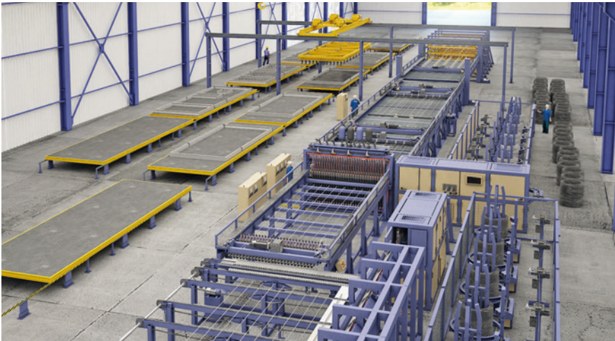
PLC AMM line with integrated universal bending modules, mesh buffer racks and distribution system on circulating pallets
