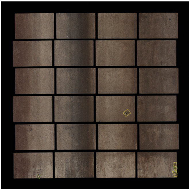
Results screen 'Defects': Each defect type is given a different colour coding.
