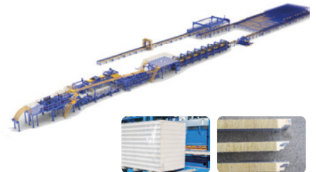
▶ YZ-100 Continuous PU/Rock wool sandwich panel production line ◀
