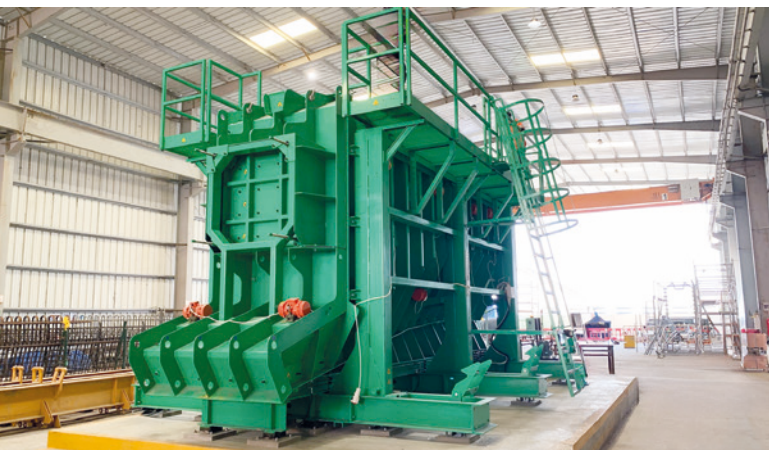
Hydraulic mould for bridge piers
