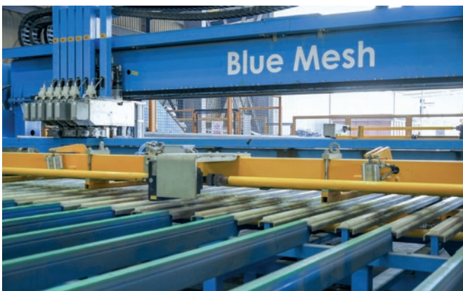
Automated mesh welding reduces waste while boosting speed and quality of the products.
