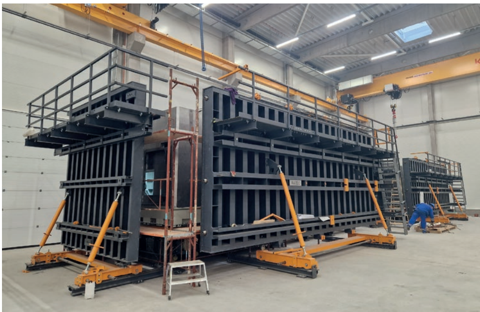
Adjustable mould for elements from 3.00 to 8.00 m in length
