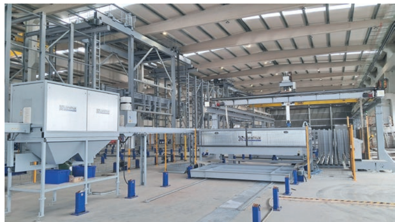
Pallet cleaning/oiling device and Shuttering cleaning/oiling device
