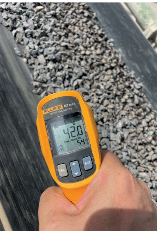
Measured inlet aggregate temperature: 42°C, production throughput 70-100 tph.
