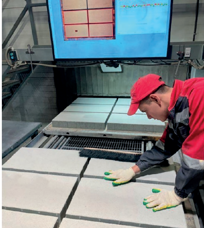
Detection of defective products on the dry side.
