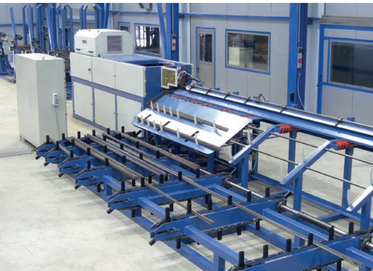
MELC Flexiline machine with order sorting pocket system
