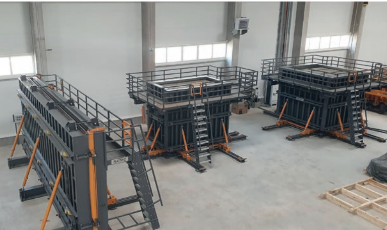
View of the factory, here with 2 modular moulds, a vertical roof mould and variable basement mould (right)
