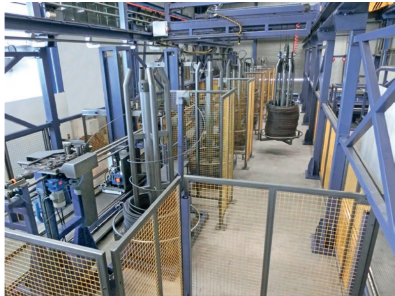
MELC Polyline NS - Automatic coil loading with robotic crane system
