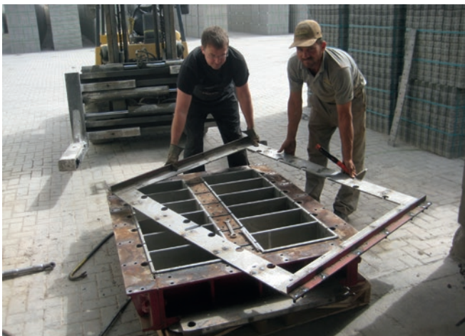
Kobra service for changing wearing parts on site
