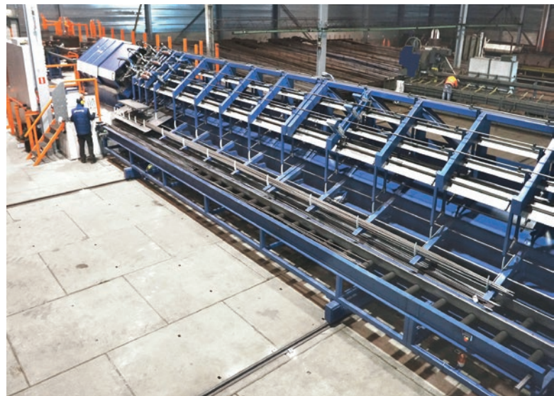
MELC Polyline with three rotors up to 25mm and coil opener robot
