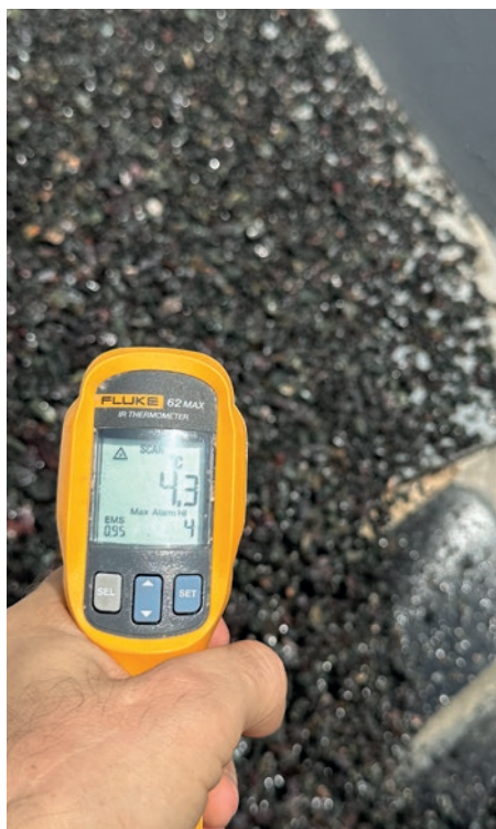
It is a matter of minutes for aggregates to exit the HydroSpiral at temperatures between less than 5 and 10 °C.
