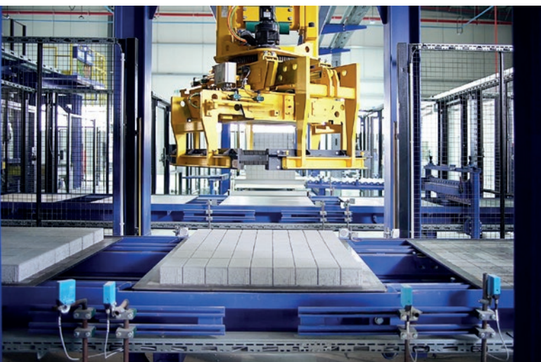
Dry side I with Cuboter: fast handling and accurate packaging of the uni products.
