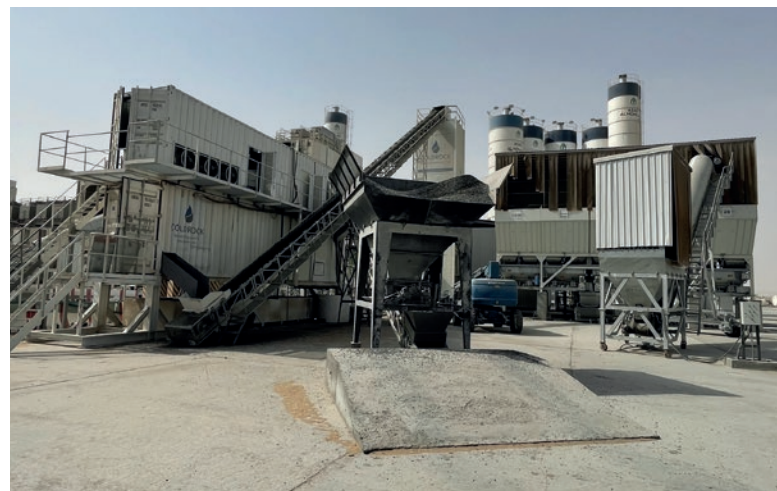
ColdRock installation complete with 80-ton insulated cold aggregates silo, NEOM jobsite in Saudi Arabia.
