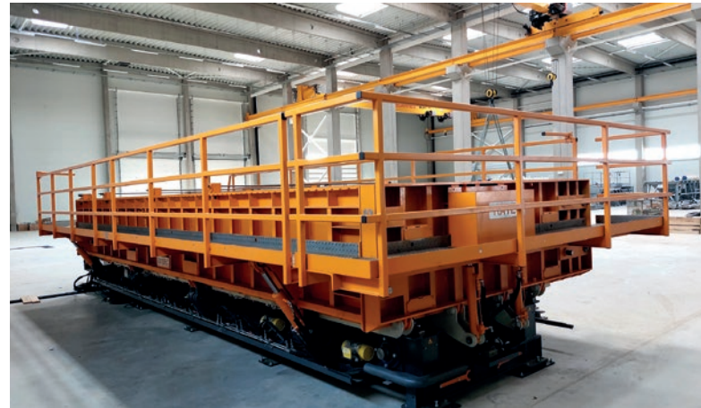
View of the factory, here with 2 modular moulds, a vertical roof mould and variable basement mould (right)
