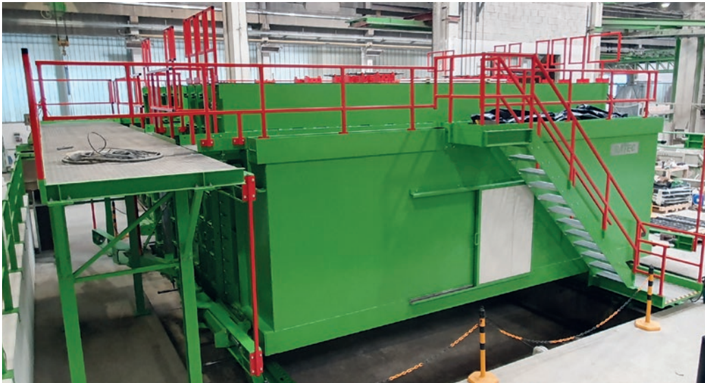
Battery formwork with platforms and stair-case
