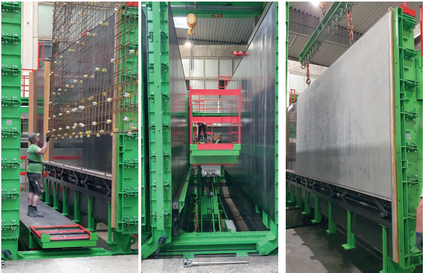
Work on the panels is made more user-friendly by the scissor-type lift platform
