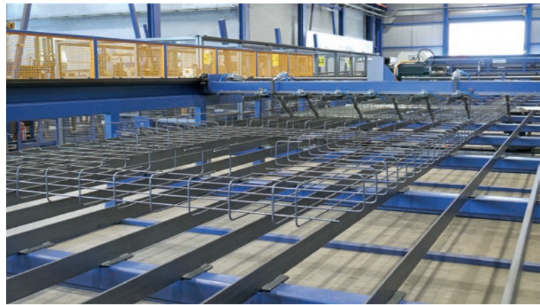
PLC AMM line with integrated universal bending modules, mesh buffer racks and distribution system on circulating pallets
