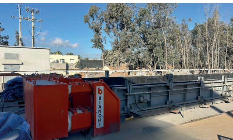
Strands anchoring structure
