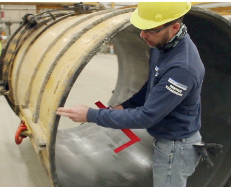
Afinitas technician performs a form maintenance check.
