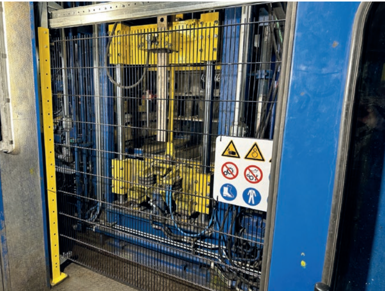
Maintenance-friendly protection of the machine by sliding door on the operator's side.
