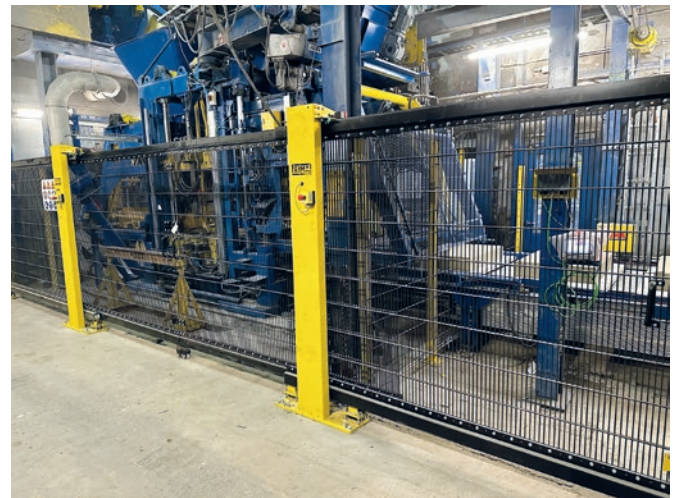
Safety sliding gate system for maintenance-friendly system protection on the mould change side.
