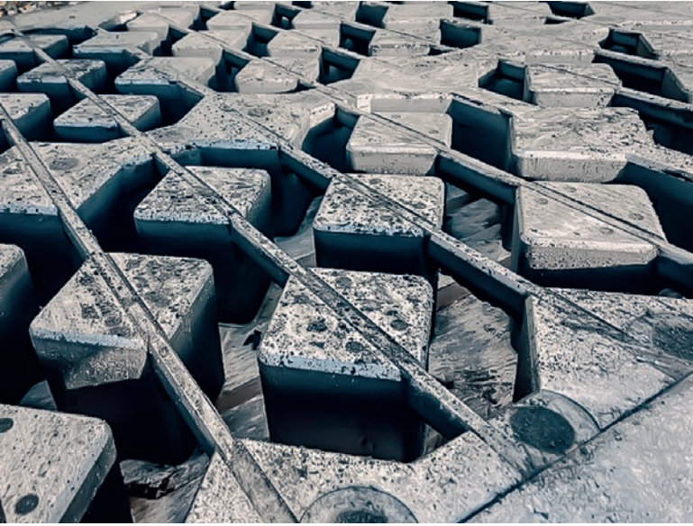
Printed cores without weld seam in mold insert
