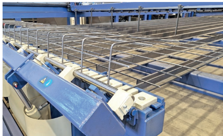
Cage production with integrated, in-line mesh bender
