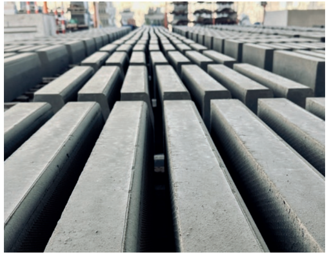
Kerbstones are produced using the wet casting process in accordance with the legal requirements of the UAE.
