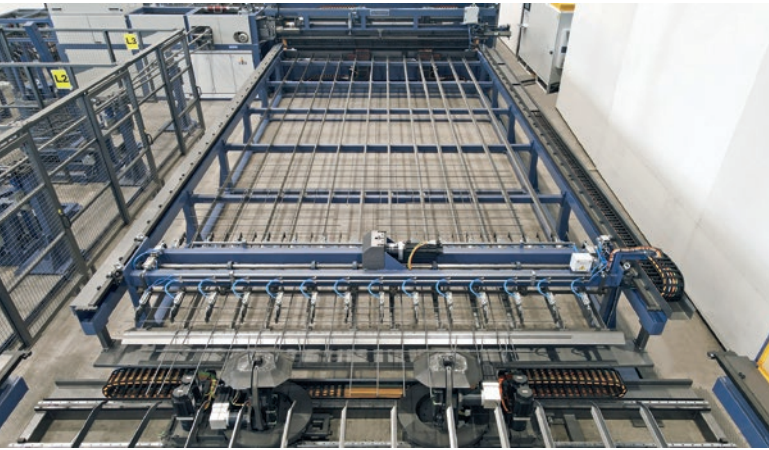
View of a PL XY machine with two integrated, in-line universal bending modules
