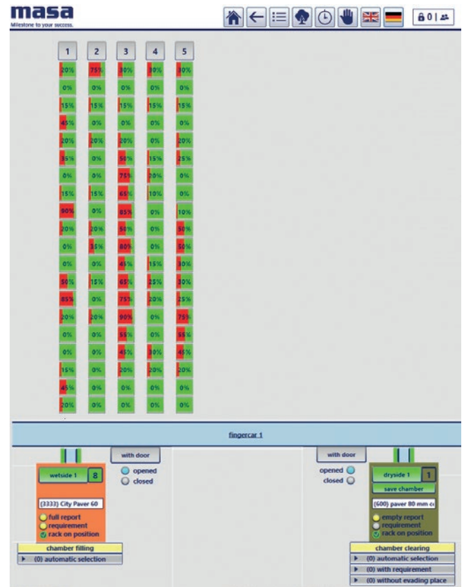
Chamber preview with visualisation of the percentage of rejects per production board
