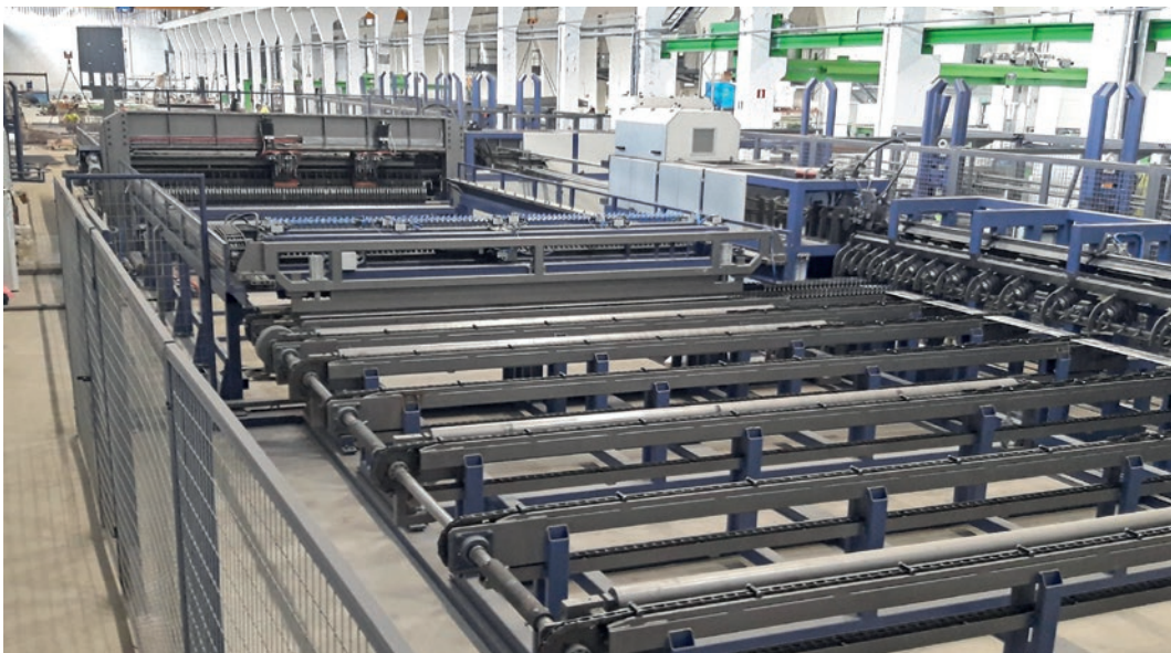
View of a PL XY AMM machine with two moving, multi-point welding heads
